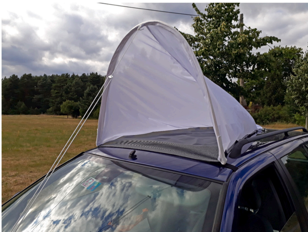
Fig. 1. An insect net installed on the roof of a car for the 'InsectMobile' project. Photo credit: S. Hecker.
